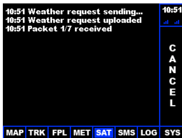
Figure 27 Transmission log screen
