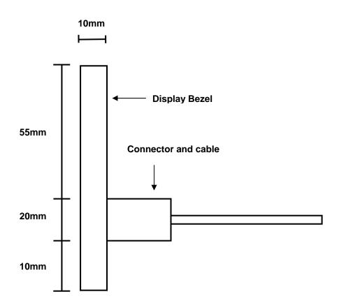
Figure 2 - Side view of external screen
