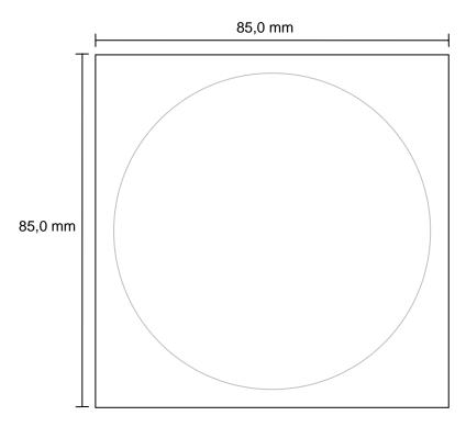
Figure 1 - Front dimensions of external screen
