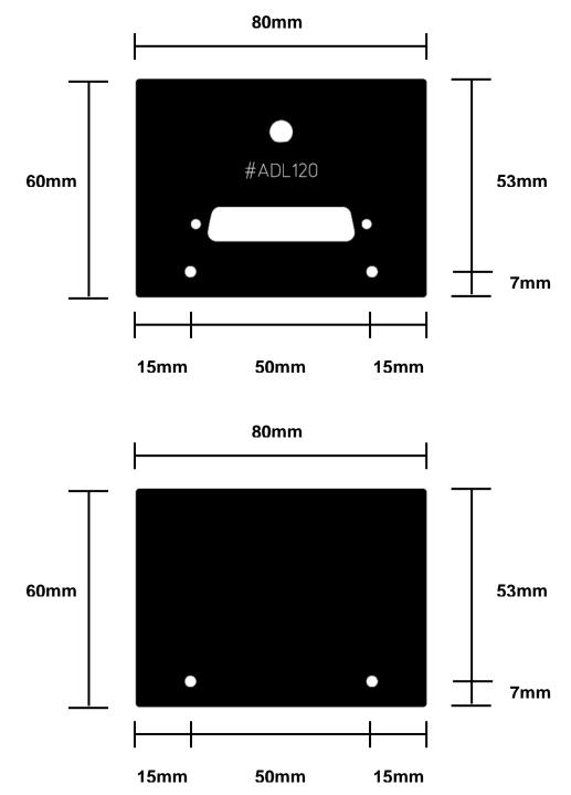
Figure 2 - Location of the M4 threads on the front and back side of the ADL120
