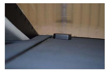
Figure 5 – Iridium SYN7391-C antenna on glareshield
